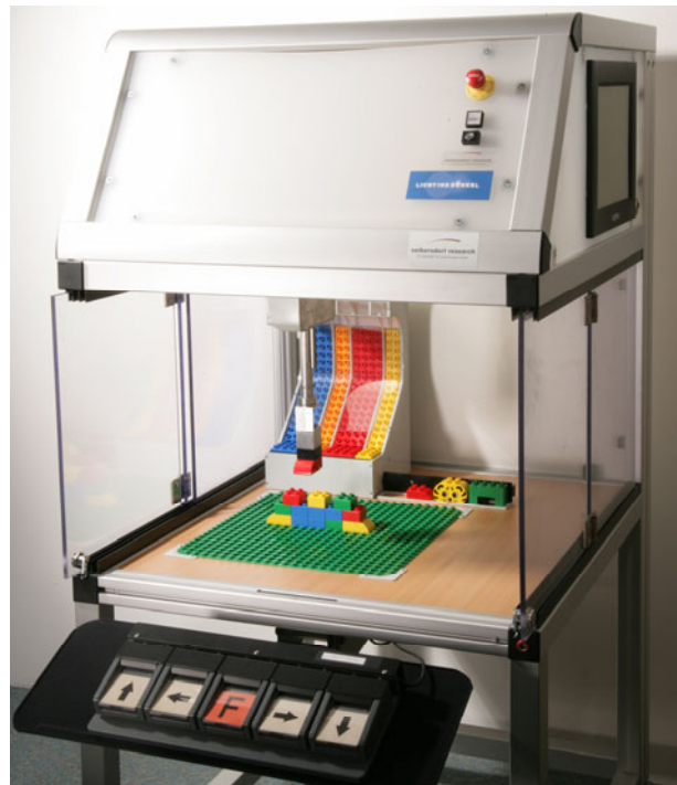
Fig. 2: Robot system “PlayROB”. The system is mounted to a mobile rack; most of the moving parts are hidden behind a cover in order to improve system safety.
