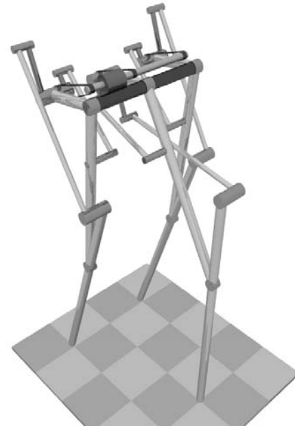
Fig. 1. 3D rendering of a single-DOF biped. The biped's design results in the need for only a single actuator. Since the biped is planar, frontal plane stability is ensured by including a third leg whose motion is slaved to the motion of the other outer leg. Note that the inertial properties of the outer two legs combined must match those of the inner leg.
