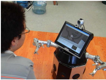
Fig. 12. Sobot User Interaction through Mobot, the Sobot has downloaded itself onto Mybot to enable monitoring of the user and thus providing anyplace and anytime service.
