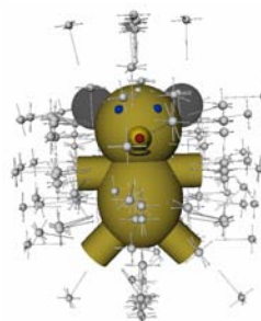
Fig. 2. Approach vectors and hand orientations representing a sampling of the grasp subspace G for a complex object composed of many superquadrics.
