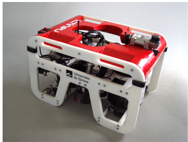
Fig. 1. ICTINEU AUV , the VICOROB-UdG Team's entry for the SAUC-E 2006 competition.
