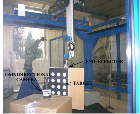
Fig. 3. Experimental setup : eye-to-hand configuration
