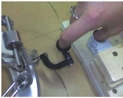
Fig. 6. The experimental setup. The figure shows the fixed thumb thimble as well as the index thimble mounted on the extremity of the haptic device via a cardanic joint. A screen (not shown in the picture) hid the view of the experimental setup to the subjects.
