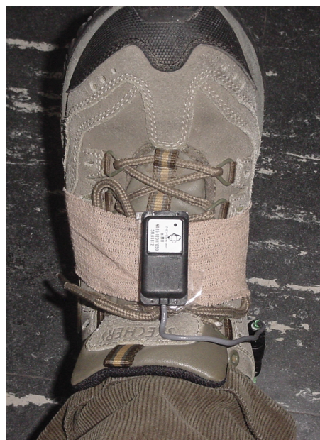
Figure 7. MemSense nImu mounted on foot for position tracking during walking, side stepping, and running.
