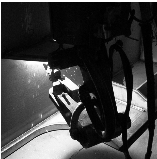
6: Hirobo WR-L80 manipulator at work at Odense Steel Shipyard.
