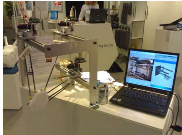
Fig. 2. Table-sized Gantry-Tau prototype shown at the Scandinavian Technical Fair (Stockholm, 3-6 October, 2006). End effector, linear tracks, and gearboxes manufactured inhouse. Drive systems from the Faulhaber Group [6]. Robot controlled from the Visual Components 3DCreate tool (laptop).
