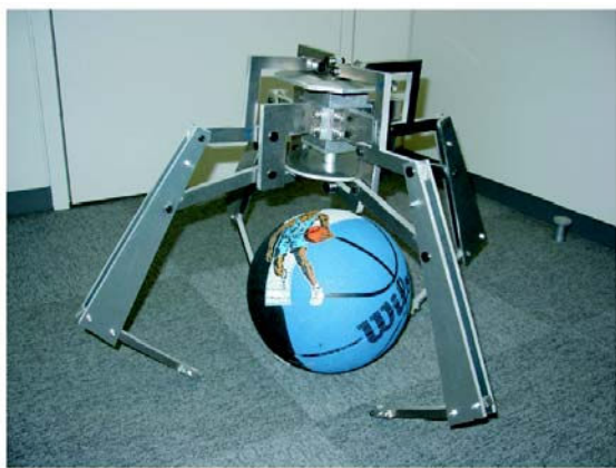
Fig. 13. Appearance of the proposed hand (No.3).
