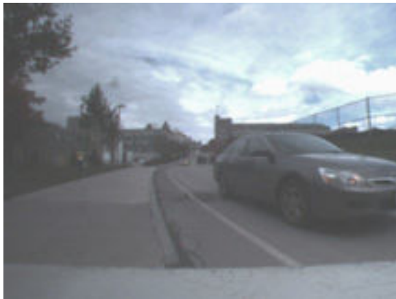
Fig. 5. An optical camera view of the roadside scene observed by the laser rangefinder (LIDAR). In this experiment the LIDAR is used to track occluded edges of obstacles. The LIDAR's x-axis lies perpendicular to the image plane, its y-axis is in the image plane to the left, and its z-axis completes the right-handed coordinate system.
