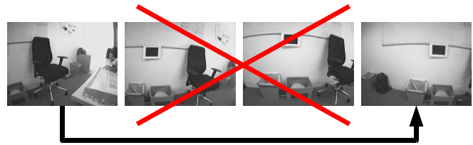
Fig. 5. To test the recovery module, sudden motion was simulated by removing the intermediate frames as the camera panned left from the image on the left to that on the right.
