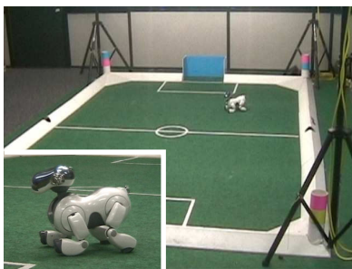
Fig. 3. The Aibo robot and its environment. Noise in the robot's joints and a relatively low resolution camera make accurate localization a difficult task.
