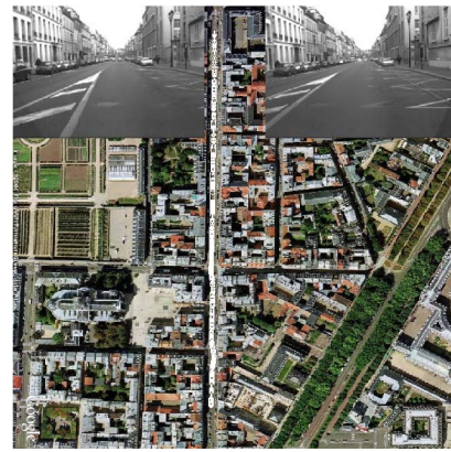
Fig. 4. Trajectory tracking around along a road in Versailles. The trajectory shown in white has been superimposed on a satellite image. A typical stereo image is shown at the top.
