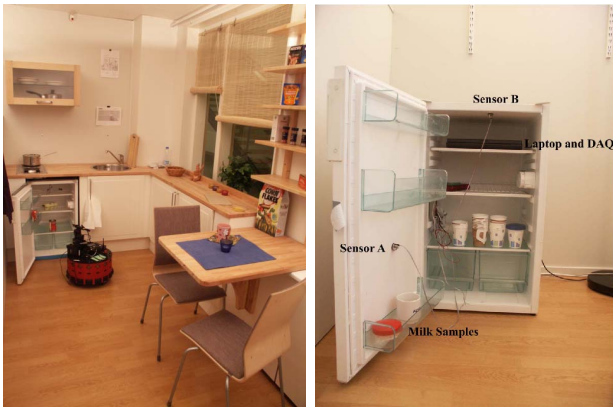
Fig. 4. (Left) Pippi is about to smell inside the fridge. (Right) The PEIS fridge showing the placement of the two gas sensors and the products to be sampled.
