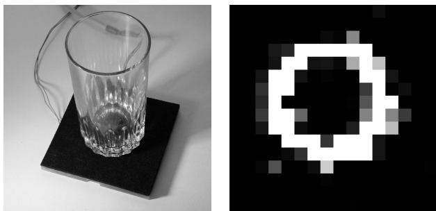
Fig. 1. On the left the sensor panel with RS-232 and power cables. An ordinary glass as seen on picture produces a pressure profile as can be seen on the right
