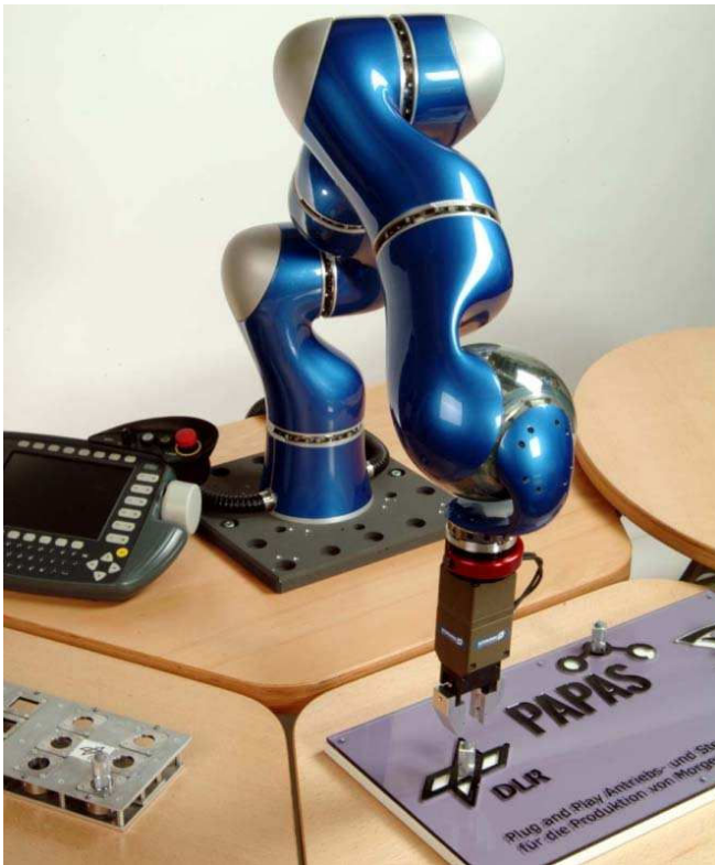
Fig. 7. Experimental setup for the assembly task using the DLR light-weight robot.
