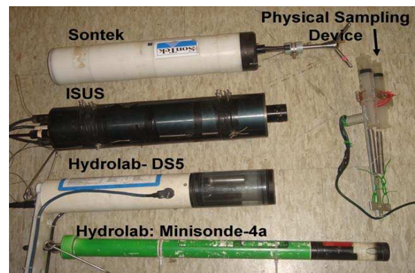
Fig. 2: Complete set of sensors with physical sampling device
