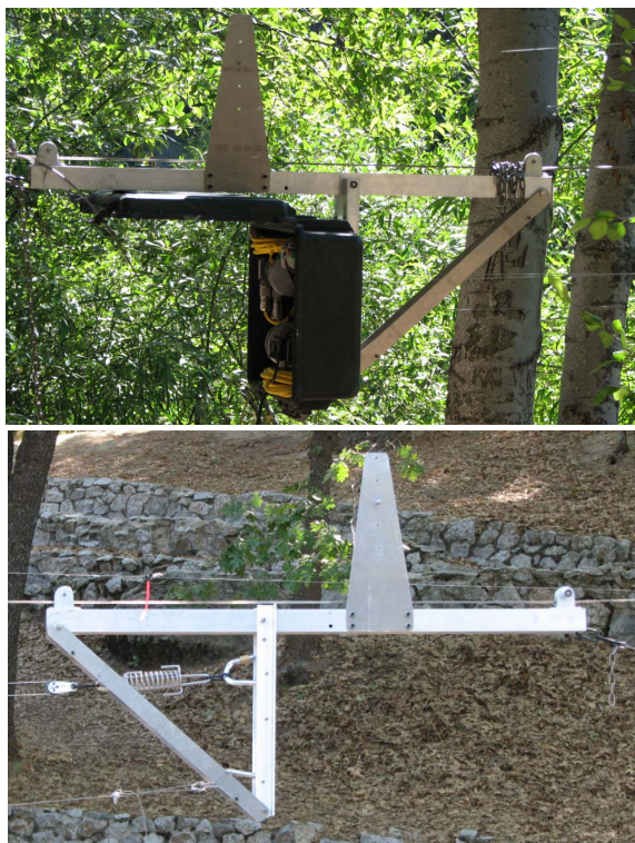
Fig. 4. These photos show the actuation module attached to one hanging anchor (top) and the cables and spring tensioner mounted to the other (bottom).
