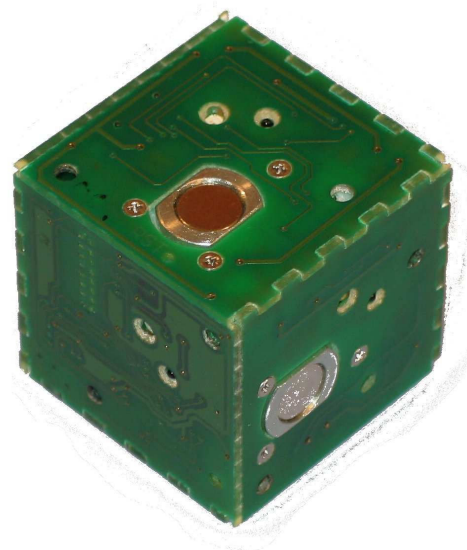
Fig. 2. Each module in the system is a cube which measures 1.77 inches on each side and weighs 4.5oz. Each module is completely autonomous and can operate for several hours under its own power.
