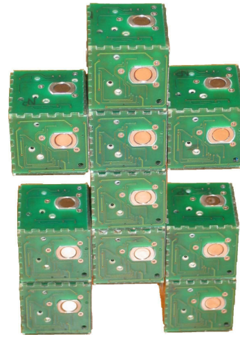
Fig. 9. The final robot-like shape we “self-disassembled” using an initial 3-by-5 rectangle of modules. From start to finish, the self-disassembly process required a total of approximately 90 seconds excluding any time spent modeling the desired final shape.
