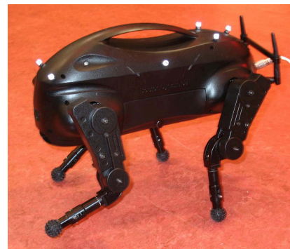
Fig. 1. LittleDog Robot A picture of the littledog robot, executing the task of keeping its center of mass over the centroid of its support polygon, while moving the front-left foot in a fast Figure-8 trajectory. The robot has a 6 axis IMU and encoders at its 12 actuated joints as well as Vicon motion capture system for body position / orientation. The body weighs 1.8kg, and each leg weighs .25kg; The body is 20cm in length, while the upper arm is 8cm, and the lower arm is 10cm.
