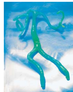
(d) Patient-specific blood vessel PVA mold constructed by dip-coating
