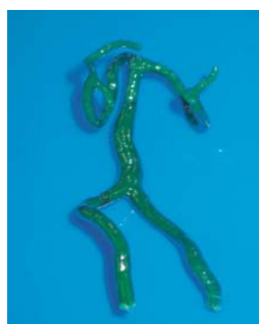
(c) Patient-specific blood vessel resin mold constructed by rapid prototyping
