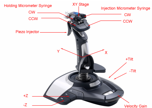
Fig. 3. Joystick function assignments: (1) translate the injection pipette along the X-, Y-, Z- and T-axis, (2) translate the XY stage along its X- and Y-axis, and (3) control the piezo-injector and micrometer syringes.
