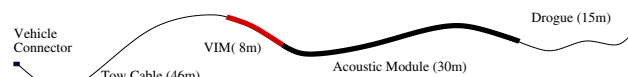
Fig. 9. The vector sensor array is roughly 100 meters in total length composed of four sections leading out from the AUV: a 47 meter tow cable section, an 8 meter vibration isolation module, a 30 meter acoustic module, and a 15 meter drogue at the end.
