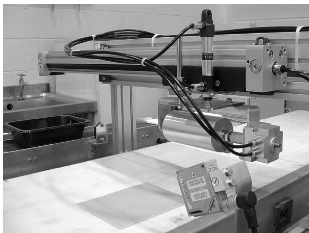
Fig. 7. Automated machine for lasagna pasta handling during trials.
