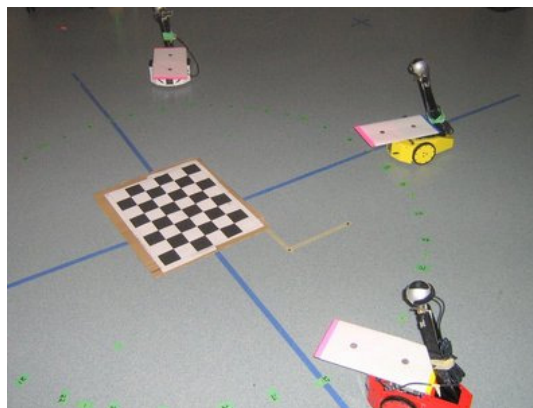
Fig. 7. The experimental setup in which a network of three mobile robots with webcams are tracking a target (checkered board)
