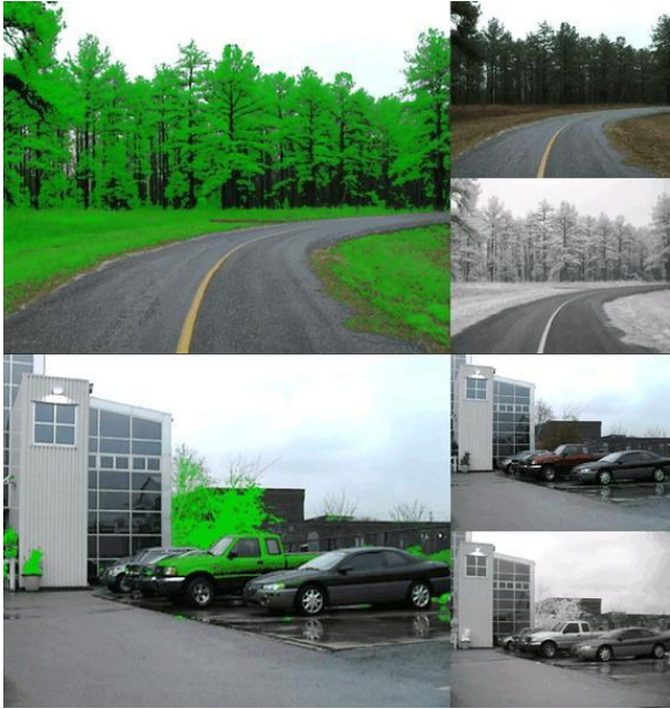
Fig. 3. Small images show the RGB and color appearance of two scenes. Large images are the RGB image with areas of high NDVI highlighted in bright green. While generally reliable in natural scenes, NDVI can fail on synthetic materials such as the paint on the truck in the right image. In this case 3-D methods would easily classify the side of the truck as a rigid obstacle instead of vegetation. Note that NDVI correctly classifies the brown dead grass in the left image as vegetation.
