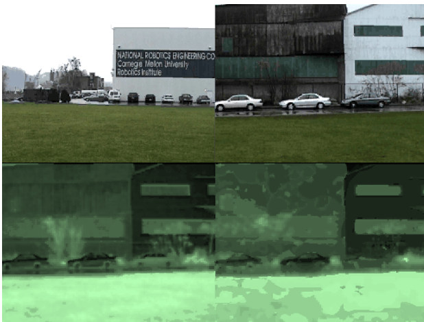
Fig. 7. NDVI can be predicted from RGB for a given environment and illumination condition, meaning the benefits of NDVI can be captured even if the NIR sensors on the robot have a much more limited field of view than the RGB sensors. The 4-color image (RGB & NIR, only RGB shown) at top left is used to train a classifier that predicts the NDVI image (bottom right) for the RGB image at top right. The ground truth NDVI image is shown at bottom left. Note how the vegetation behind the cars is detected against the dark green portion of the building.
