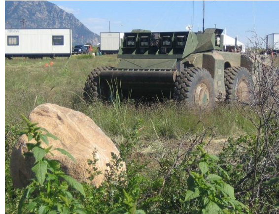
Fig. 1. Autonomous mobile robot used for this evaluation. The addition of NIR data helps in discrimination between the rock on the left and the bush on the right.
