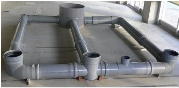
Fig. 17. Our test field, including all kinds of pipe bends, small steps and also navigational landmarks such as manhole, inlets and pipe joints, can present as a sample of real world sewer network in Japan.
