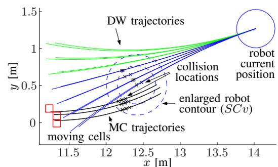
Fig. 3. Collision of MC and DW trajectories
