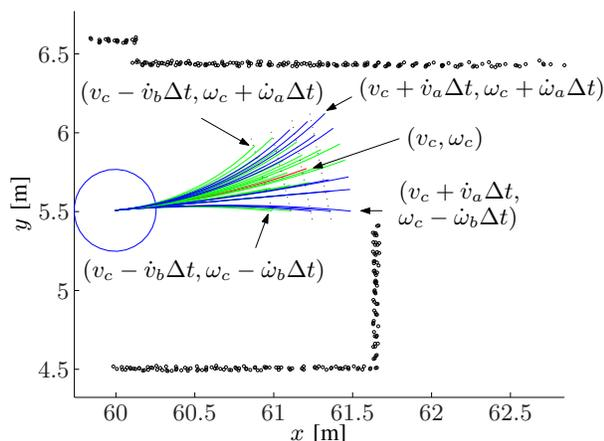
Fig. 1. A snapshot of possible robot trajectories
