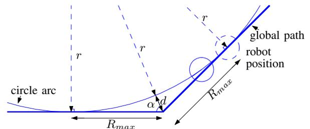
Fig. 6. Maximal robot departure from the path
