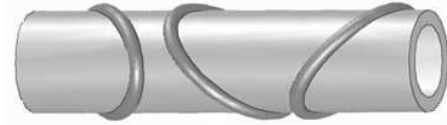
Fig. 3. Schematic of passive marker placed on a surgical instrument. The relative positions of the three bumps encode the roll angle and tip position of the surgical instrument.
