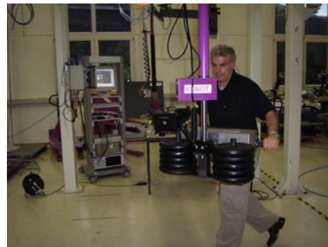
Figure 12. Railway crane admittance display with 100 kg payload
