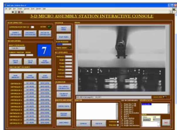
Figure 3: GUI for \mu^3 showing video feed of a MEMS part approximately 500 \mu\text{m} tall gripped by a milli-nozzle
