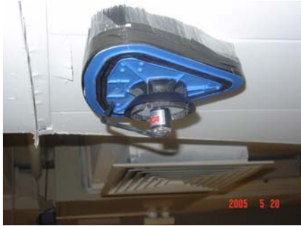
Fig. 3 The City-Climber V1 clings to a ceiling.
