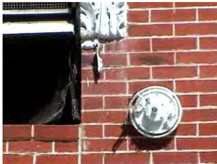
Fig. 4 City-Climber V2 approaching a window on brick wall; while transmitting real-time video for inspection purpose
