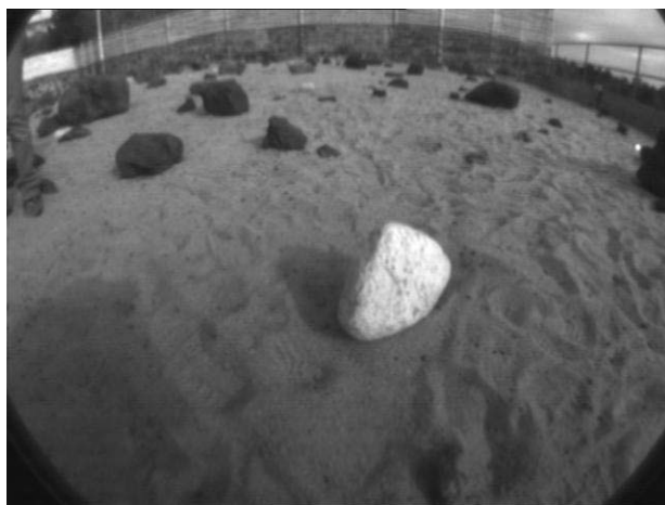
Fig. 5. Image taken in response to a science alert on the JPL FIDO rover. In this test, science alerts were generated for “high albedo” (or light-colored) rocks.
