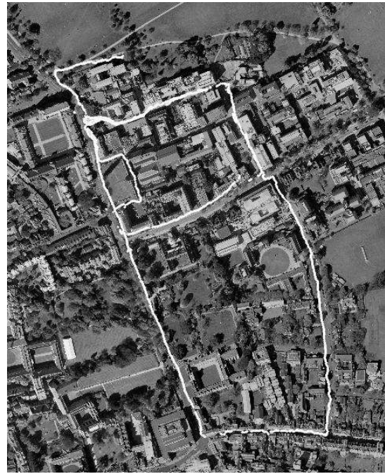
Fig. 3. An aerial map of the Oxford Science Park data set (3.3 km, 8536 images). The vehicle's trajectory is marked in white.
