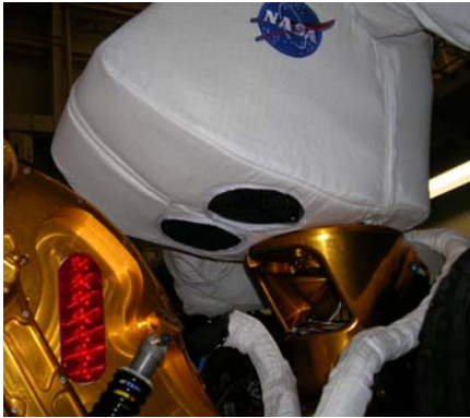
Figure 7: Filtered inlet fans at the base of Centaur's upper body
