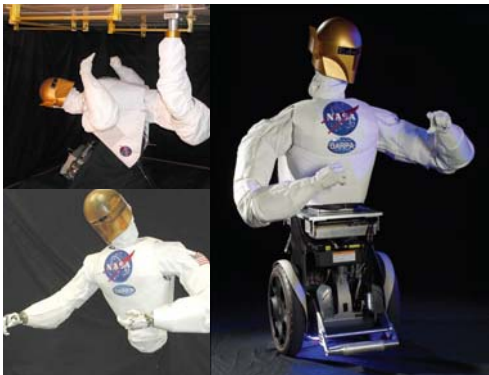
Figure 1: (counterclockwise starting at top left) Robonaut with 0g leg, Robonaut with 3 DoF waist, Robonaut on Segway™ RMP
