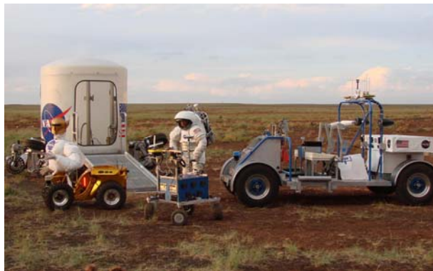
Figure 8: All four robots and a suited subject at the coordinated field demonstration in the desert. From left to right: ATHLETE kneeling (rear), Centaur, K-10 (front), suited subject, SCOUT
