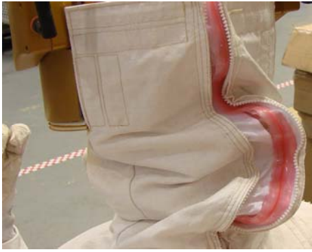
Figure 6: An opened zipper and zip-lock, anti-static, plastic seal on the back of Robonaut's neck
