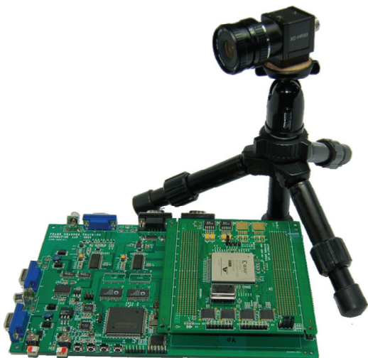
Fig. 6. A vision system employing a multiple objects tracking circuit using particle filters with multiple features.
