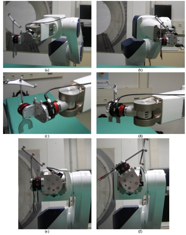
Fig. 4. Episodes of the automatic end-effector registration procedure. (a)-(b) Movement along the y-axis of the robot. (c)-(d) Positions for rotating the end-effector in the xz-plane of the flange coordinate system. (e)-(f) Start and final location of the rotation in the xy-plane.
