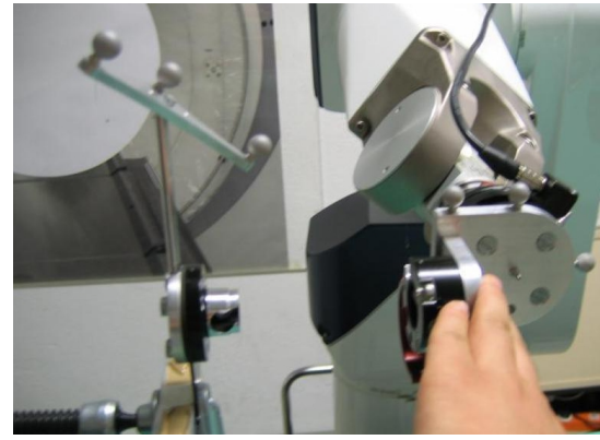
Fig. 6. By applying forces and torques to the end-effector base (right), the coupling motion towards the mouth piece (left) is induced by the user.
