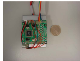
Fig. 4. Circuit board together with battery
