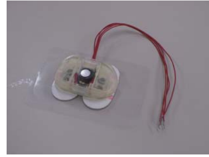
Fig. 11. Probe for bioelectric potential (built-in instrumentation amplifier)
