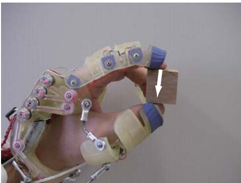
Fig. 14. Grasping force direction during pinching: Arrow means direction of the assistive force(from index fingertip to tip of thumb) when the index fingertip is further than tip of thumb from a palm. The direction becomes from index fingertip to a MP of thumb if the index fingertip is nearer than tip of thumb from a palm.
