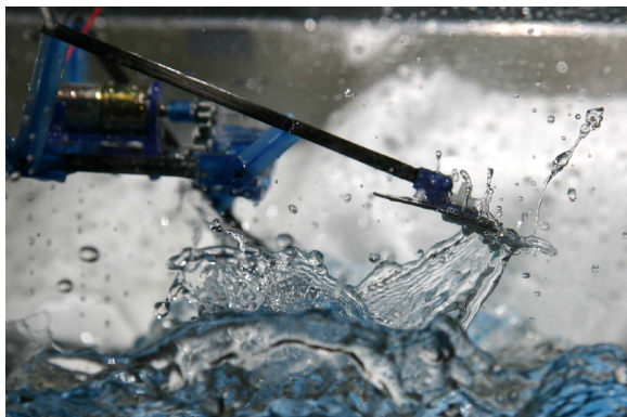
Fig. 3. Photograph of the water plume dragged from the cavity by the foot during the retraction phase of the robot's step.
