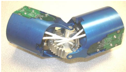
Fig. 2. Joint angular actuator with onboard electronics.
