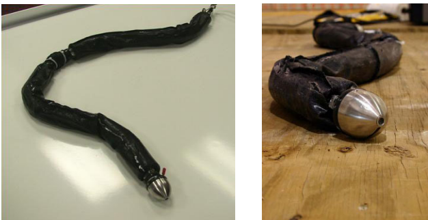
Fig. 3. The 156cm integrated TSD test system used for experiments.
