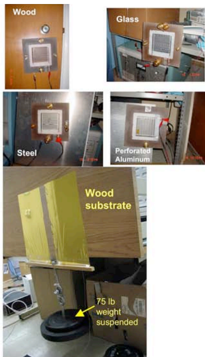
Fig. 2. Electroadhesive pads clamping and holding weights up on various surfaces.
