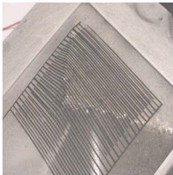
Fig. 3. Prototype electroadhesive pad conforming to a rough (concrete) surface.
