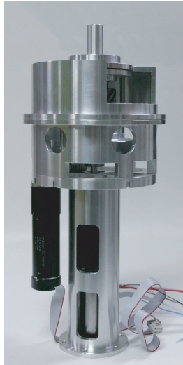
Fig. 4. Implemented VSJ. It consists of two motors and VSU.
