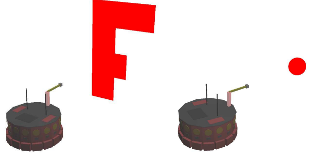
Fig. 2: Webots simulation environment with a mobile manipulator carrying a camera mounted on the end-effector. As target objects, we considered the case of a planar ‘‘F’’ shape (left) and of a sphere (right).
