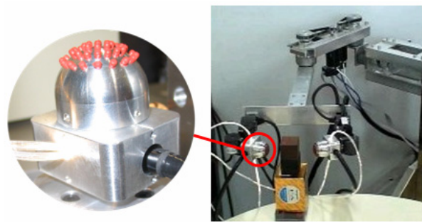
Fig. 2. Multi-fingered humanoid robot arm mounted with optical three-axis tactile sensors at fingertips.
