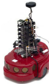
Fig. 5. Amigobot rover with custom subsystems
