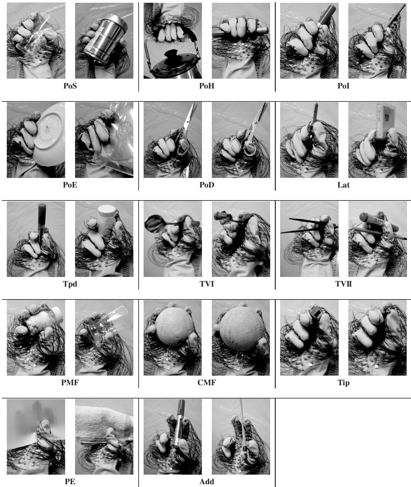
Fig. 6. Photographs of Kamakura's grasp types with the Cyber Glove and the tactile sensing glove.
