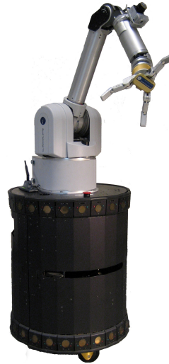
Fig. 5. UMan (UMass Mobile Manipulator)
