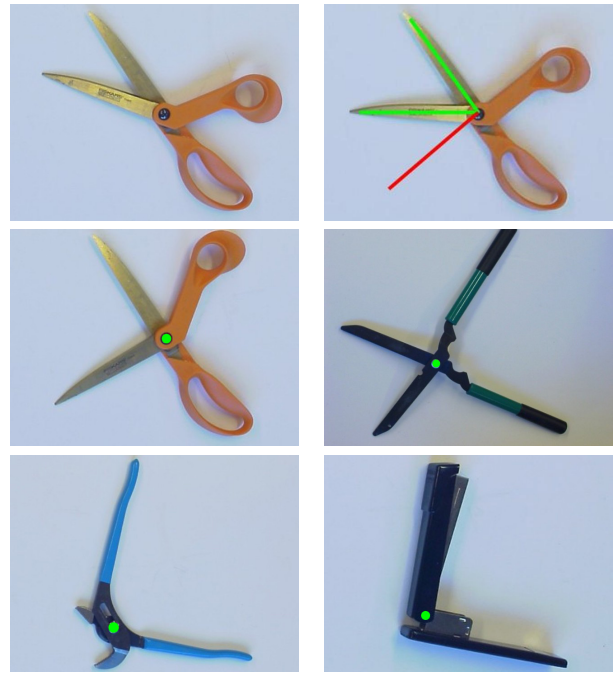
Fig. 6. Experimental results showing the manipulation of articulated objects based on interactive perception. The first row shows the scissors before the interaction (left) and after the interaction (right). The right image also illustrates the generated manipulation plan for forming a 90^\circ angle between the blades. The remaining images show the detected revolute joints (marked with a green dot), and the results of executing the respective manipulation plans for forming a 90^\circ angle between the objects' links. The scale of objects varies from 15cm (stapler) to 50cm (shears) in length.
